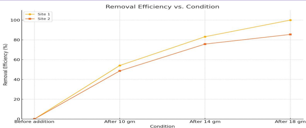
Fig. 1. Heavy Metal Removal Efficiency Using Biopolymer in Contaminated Oily Soil – Site 1
