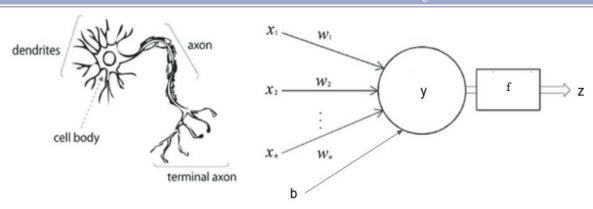
Where  $x_1,...,x_n$  are the inputs,  $w_1,...,w_n$  the corresponding weights and b as bias.
