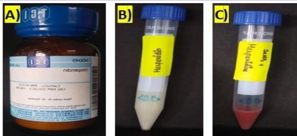
Figure 3: Preparation of hesperidin–SeNP nanoformulation. (A) Hesperidin powder; (B) Preparation of stock solution; (C) Incorporation of SeNPs with hesperidin, indicated by a distinct color change.
