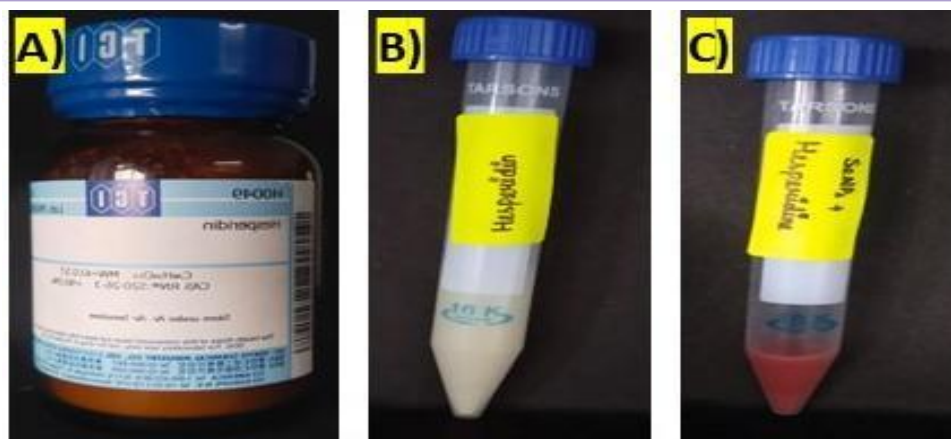
Figure 3: Preparation of hesperidin–SeNP nanoformulation. (A) Hesperidin powder; (B) Preparation of stock solution; (C) Incorporation of SeNPs with hesperidin, indicated by a distinct color change.
