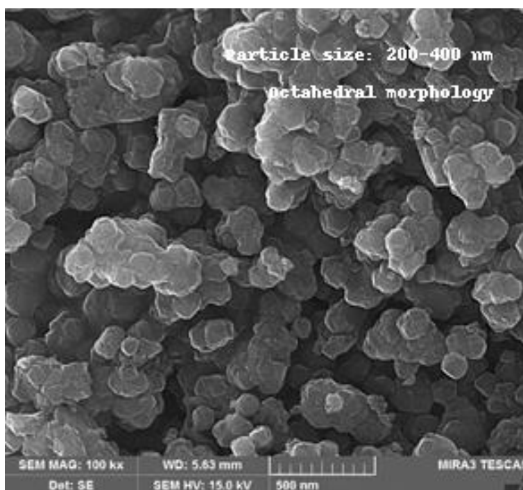
Figure 3. SEM images showing morphology of pristine UiO-66-NH 2 and magnetic composite at different magnifications.
